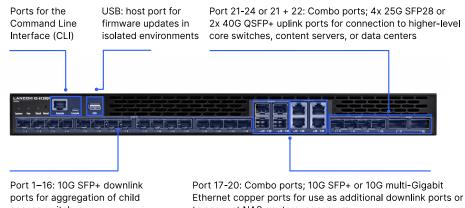
Figure 6a: LANCOM XS-6128QF port layout (front)
