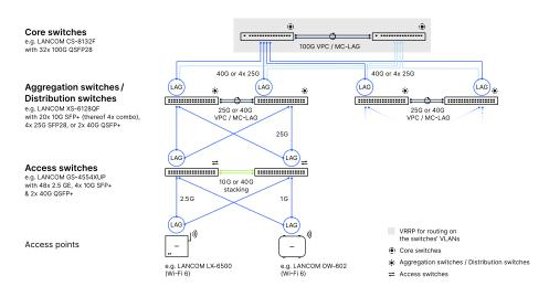
Figure 3: Scenario with a combination of VPC and stacking
