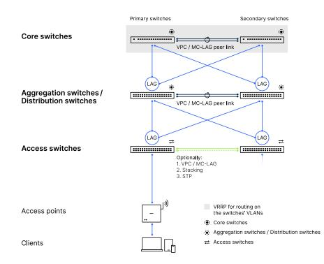
Figure 1: Three-tier network with redundancies
