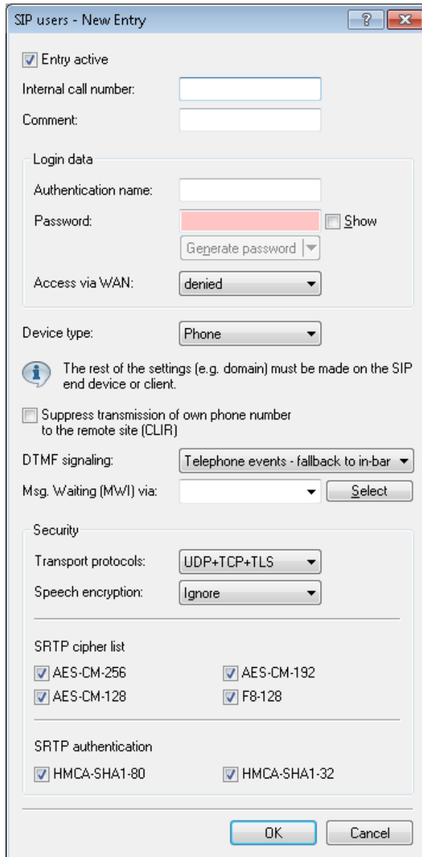
Figure 35: Adding a new entry to the SIP user table
