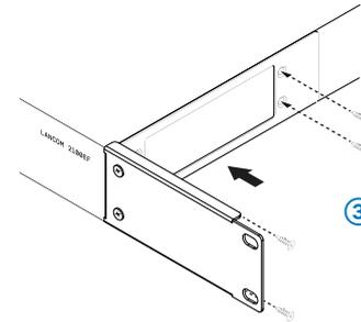
The Rack Mount 2100 kit consists of 2 mounting plates ① and ② for each side of the device, which are first connected to each other with 2 of the enclosed screws ③ to form 2 mounting brackets, before these are attached to the device and rack with the other screws.
